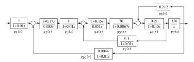
**Figure 2.4.** An example of DC electric drive system.
