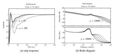
**Figure 7.5.** Closed-loop system responses with different p.
