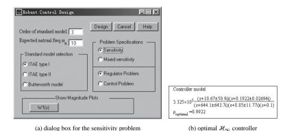
**Figure A.45.** Robust control design results.
