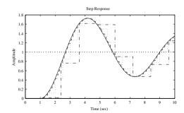
**Figure 3.9.** Step response comparisons of discretized systems.
