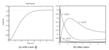
**Figure 5.17.** *Step responses of closed-loop systems.*
