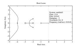
**Figure 3.16.** *Root locus for positive feedback systems.*
