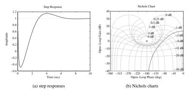
**Figure 7.21.** System responses with an  $\mathcal{H}_{\infty}$  controller.
