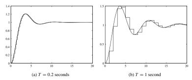
**Figure 4.21.** Step responses for different sampling intervals.
