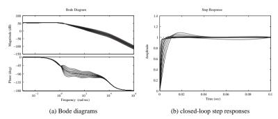
**Figure 8.9.** Time and frequency domain analysis under robust controller.
