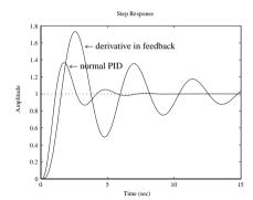
Figure 6.10. PID controllers comparison.
