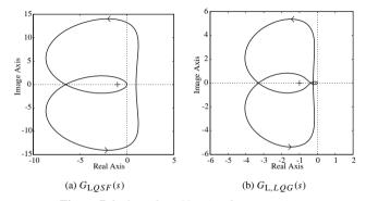
**Figure 7.6.** Open-loop Nyquist plot comparison.
