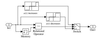
**Figure 4.32.** *Double-valued relay nonlinearity (file: c4mloop.mdl).*
