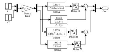
**Figure 4.17.** Simulink model of the multivariable system (c4mmimo.mdl).
