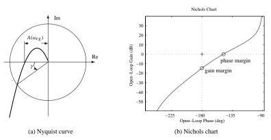
**Figure 3.26.** *Graphical representations of gain and phase margins.*
