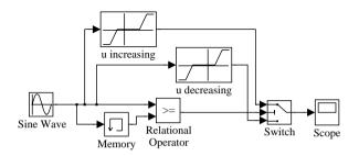
**Figure 4.34.** *Simulink model for sinusoidal distortions (file: c4msin.mdl).*
