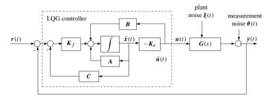
Figure 7.2. LOG control structure.
