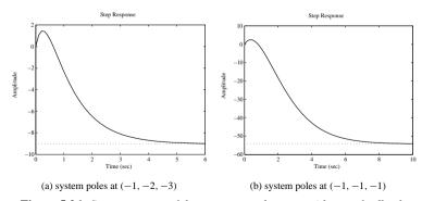
**Figure 5.26.** Step responses of the compensated system with state feedback.
