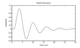
Figure 3.11. Impulse response of the system.
