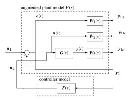
**Figure 7.14.** *Two-port diagram with weighting functions.*
