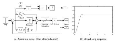
**Figure 8.10.** Optimal PID controller design for fractional-order plant.
