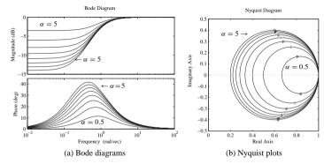
**Figure 5.2.** Frequency domain representation of a lead compensator.
