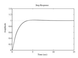
Figure 8.8. Integer-order PID control of fractional-order plant.
