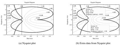
**Figure 3.21.** Nyauist plot analysis of the system in Example 3.30.
