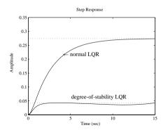
**Figure 5.19.** *Step responses of the closed-loop systems.*
