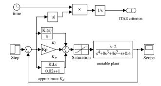
**Figure 6.33.** Simulink model for PID control (file: c6munsta.mdl).
