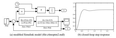
Figure 6.26. Modified simulation model and response.
