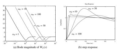
**Figure 7.33.** System responses with optimal  $\mathcal{H}_{\infty}$  controllers.
