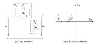
**Figure 5.1.** *Lead compensator.*
