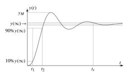
**Figure 3.6.** *Typical step response specifications.*
