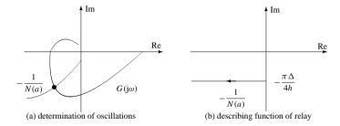
**Figure 6.41.** Determination of the magnitude and frequency of oscillations.
