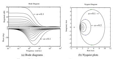
**Figure 5.6.** *Frequency responses of lag compensators.*
