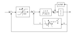
**Figure 4.9.** An example of a nonlinear system.
