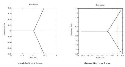
**Figure 3.19.** Problems in automatic root locus drawing.
