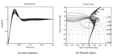
**Figure 7.24.** System responses for different  $\delta$ .
