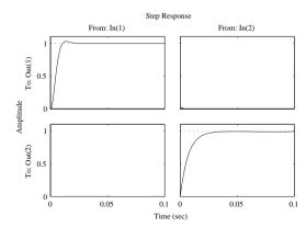
**Figure 7.25.** Step response under the optimal  $\mathcal{H}_{\infty}$  controller.
