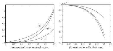
Figure 5.22. State observers of unstable models.
