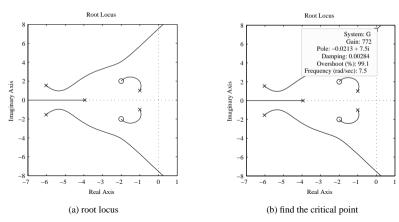
**Figure 3.14.** Root locus analysis of the system and its inverse.
