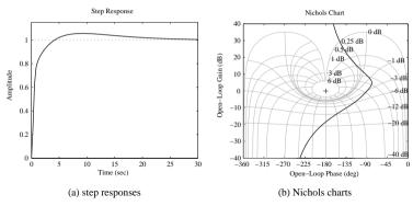
**Figure 7.23.** System responses when the poles are shifted.
