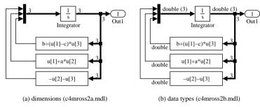
Figure 4.16. Enhancements of vector signal blocks.
