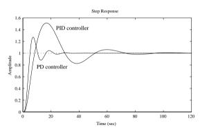
Figure 6.21. Comparisons of the PID and PD controllers.
