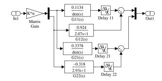
**Figure 4.40.** *MIMO Simulink model (file: c4mmdly1.mdl).*
