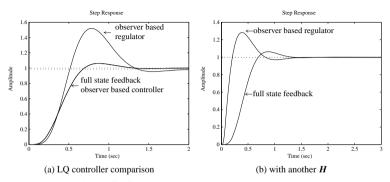
**Figure 5.25.** *Step responses of LO optimal control.*
