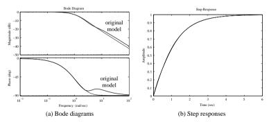
**Figure 3.29.** Bode diagram and step response comparisons.
