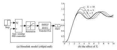
Figure 6.38. Effect of anti-windup PI controllers.
