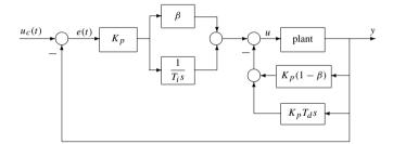
Figure 6.16. Refined PID control structure.
