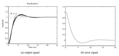
**Figure 6.4.** PID control with approximate derivatives.
