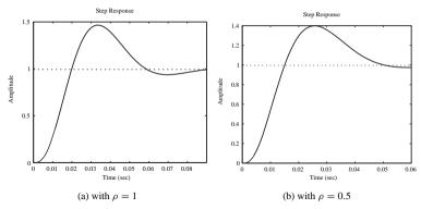
**Figure 7.19.** Closed-loop step responses for different  $\rho$ .
