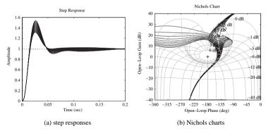
**Figure 7.27.** System responses for different  $\delta$ .
