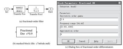
Figure 8.4. Fractional-order differentiator block design.
