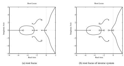
**Figure 3.20.** Root locus of a system and its inverse system.
