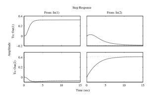
**Figure 4.18.** *Comparisons of the multivariable system simulation results.*
