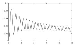
**Figure 4.28.** *Impulse response of the time varying system.*
