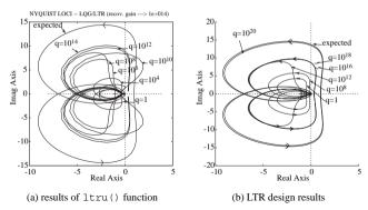
**Figure 7.10.** LOG/LTR controller design using different methods.
