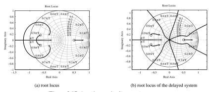
**Figure 3.15.** *Root locus of a discrete-time system.*
