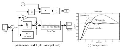
**Figure 6.30.** PID control model and response comparisons.
