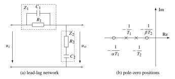
Figure 5.9. Lead-lag compensator.
