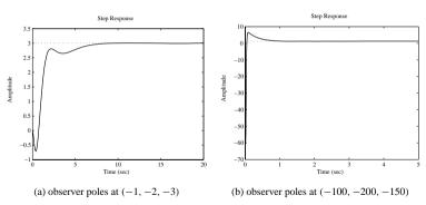
**Figure 5.27.** Step responses of observed-based systems.
