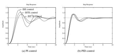
**Figure 6.18.** Closed-loop step responses of optimal controllers.
