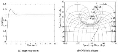
**Figure 7.31.** System responses with optimal  $\mathcal{H}_{\infty}$  controllers.
