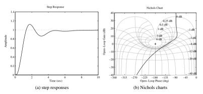
Figure 6.19. Responses for the optimal gain-phase margins design.
