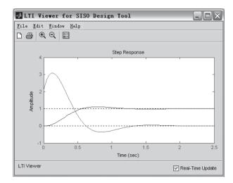
**Figure 5.31.** *Step response of the compensated system.*
