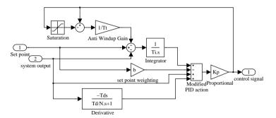
**Figure 6.37.** Anti-windup PID structure (file: c6awpid.mdl).
