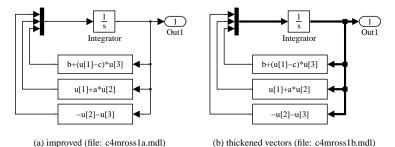
**Figure 4.15.** Another simulink description of the Rössler equations.
