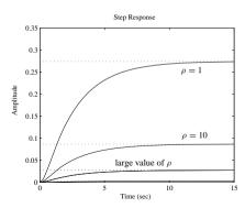
Figure 5.18. Step responses of closed-loop systems.
