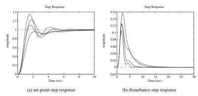
Figure 6.14. Closed-loop step responses of CHR controllers.
