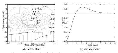
**Figure 7.28.** Dynamic behavior of a system under the  $\mathcal{H}_{\infty}$  controller.
