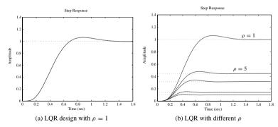
**Figure 5.15.** Step responses of closed-loop systems.
