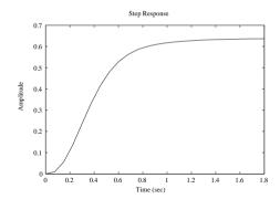
**Figure 7.22.** System responses with an  $\mathcal{H}_{\infty}$  controller.
