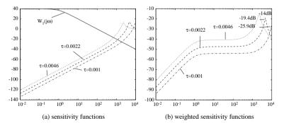
**Figure 7.17.** Bode magnitude plots for different controllers.
