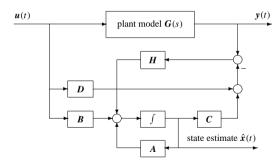
**Figure 5.20.** A typical structure of state observers.
