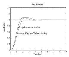
Figure 6.20. Step responses comparison of two PID controllers.
