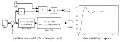
**Figure 6.25.** *Phase lead-lag controller and system response.*
