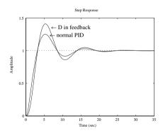
**Figure 6.6.** The closed-loop step responses comparison.
