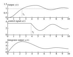
Figure 6.36. Integrator windup demonstration.
