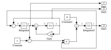
**Figure 4.13.** Simulink model of Rössler equations (file: c4mrossler.mdl).
