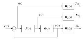
**Figure 7.13.** *Block diagram of general weighted sensitivity functions.*
