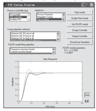
**Figure 6.24.** *PID controller design and display.*
