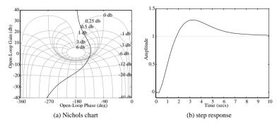
**Figure 7.29.** Dynamic behavior of a system with the optimal  $\mathcal{H}_{\infty}$  controller.
