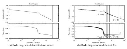
**Figure 3.24.** Bode diagrams of the discrete-time models in Example 3.31.
