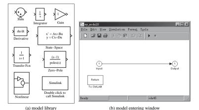
Figure A.5. Simulink model entering in CtrlLAB.
