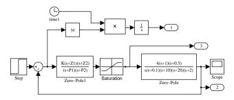
**Figure 6.27.** The Simulink model with saturation (file: c6moptm3.mdl).
