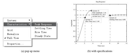
**Figure 3.7.** *Step response with specifications.*
