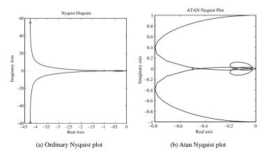
**Figure 3.27.** Transformed Nyauist plots (arc tangent).
