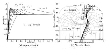
**Figure 7.32.** *System responses with an*  $\mathcal{H}_{\infty}$  *controller.*
