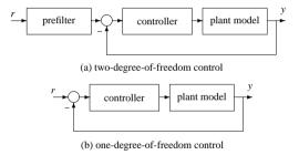
Figure 1.3. Feedback control structures.
