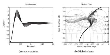
**Figure 7.20.** *System responses for different*  $\delta$ .
