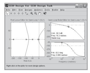
**Figure 5.29.** The user interface of SISOTool.
