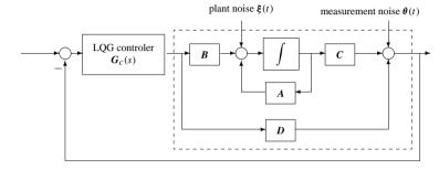
Figure 7.3. Observer-based LOG control structure.
