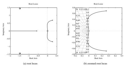
**Figure 3.17.** Root locus according to variable a.
