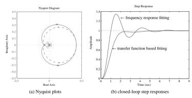
Figure 6.11. PID controller responses.
