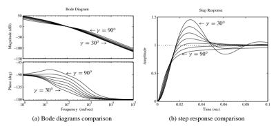
**Figure 5.11.** The effect of the desired phase margin  $\nu$ .
