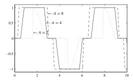
**Figure 4.35.** *Nonlinear distortion of sinusoidal inputs.*
