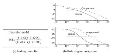
Figure A.35. A lead-lag compensator.
