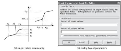
**Figure 4.29.** Construction of single-valued nonlinearities.
