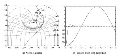
Figure A.46. Robust control system analysis.
