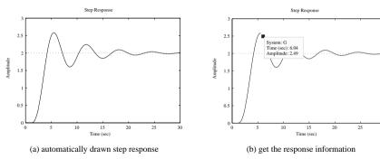
**Figure 3.8.** Step response of a delayed continuous system.
