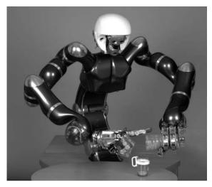
Fig. 1.33. The Justin humanoid robot manipulator (courtesy of DLR)
