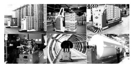
**Fig. 1.22.** Examples of AGVs for material handling (courtesy of E&K Automation GmbH)
