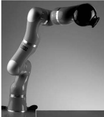
**Fig. 1.30.** The KUKA LWR robot (courtesy of KUKA Roboter GmbH)
