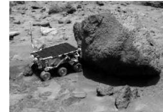
Fig. 1.35. The Sojourner rover was deployed by the Pathfinder lander and explored 250 m<sup>2</sup> of Martian soil in 1997 (courtesy of NASA)
