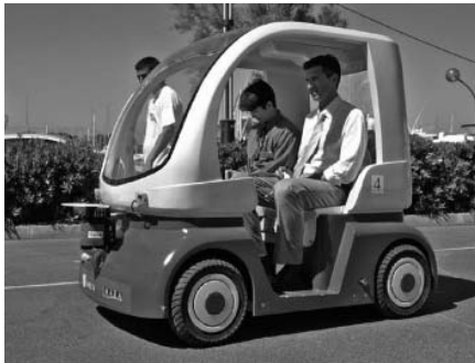
Fig. 1.37. The Cycab is an electrically-driven vehicle for autonomous transportation in urban environments (courtesy of INRIA)
