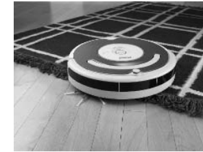
Fig. 1.39. The vacuum robot Roomba, employing a differential-drive kinematics, autonomously sweeps and cleans floors (courtesy of I-Robot Corp)
