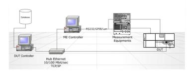
Fig. 1 The Automatic Test System Architecture. **DUT** device under test, DUT Controller, **ME** Measuring Equipments which collect and check observable values from the DUT, the ME Controller connected with the ME
