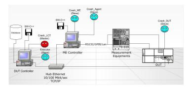
Fig. 2 The Automatic Test recovery Mechanism Architecture
