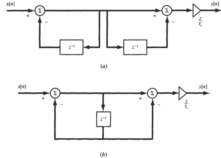
**Fig. 6-30** Simulation of a differentiator.
