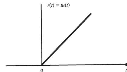
Fig. 1-34 Unit ramp function.
