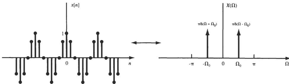
Fig. 6-15 A cosine sequence and its Fourier transform.
