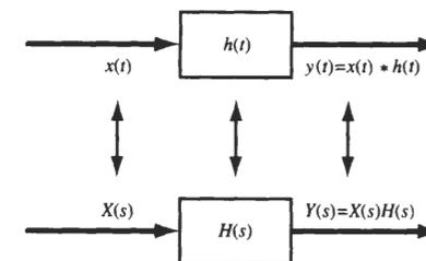
Fig. 3-7 Impulse response and system function.
