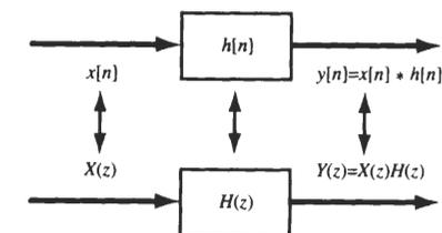
Fig. 4-3 Impulse response and system function.
