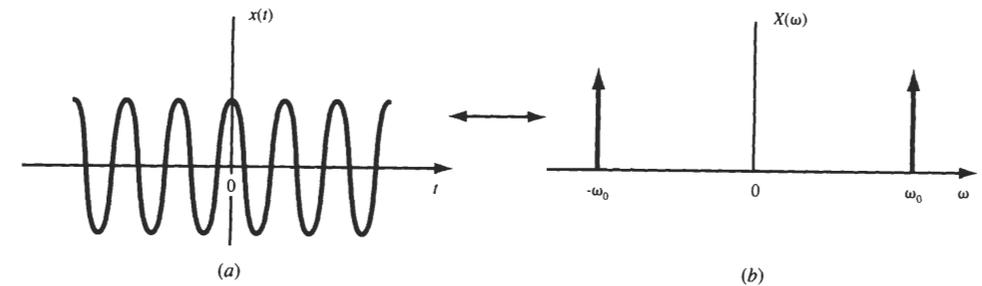
**Fig. 5-21** Cosine signal and its Fourier transform.
