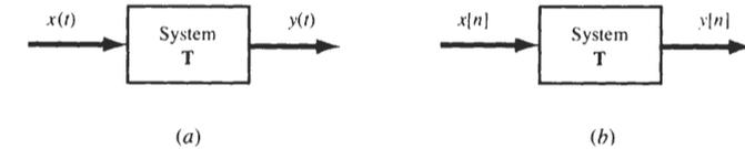
Fig. 1-15 (a) Continuous-time system; (b) discrete-time system.
