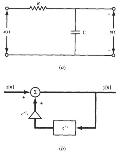
Fig. 6-28 Simulation of an RC filter by the impulse invariance method.
