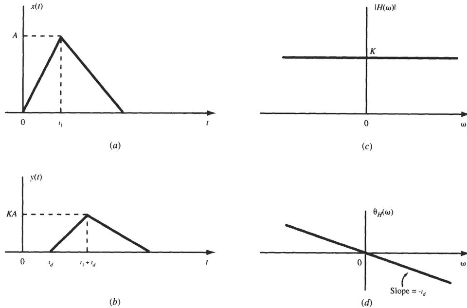
Fig. 5-4 Distortionless transmission.
