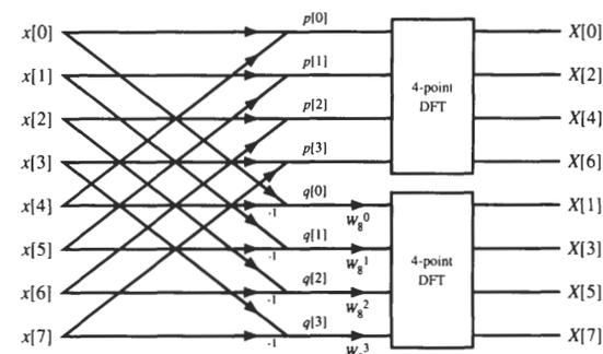
**Fig. 6-39** Flow graph for an 8-point decimation-in-frequency FFT algorithm.
