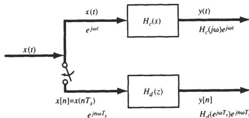
Fig. 6-5 Digital simulation of analog systems.
