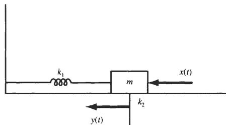
Fig. 7-4 Mechanical system.
