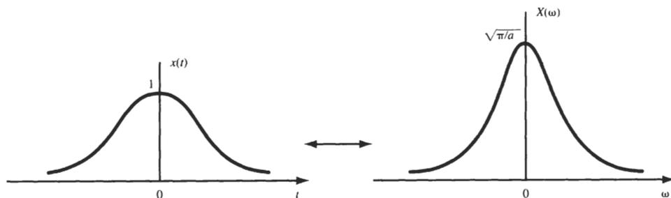
Fig. 5-26 Gaussian pulse and its Fourier transform.
