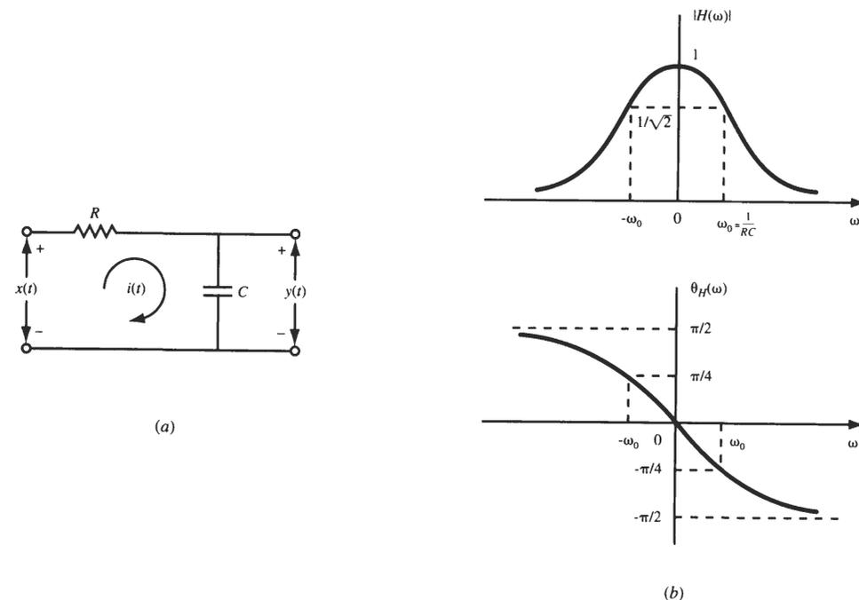
Fig. 5-6  $RC$  filter and its frequency response.
