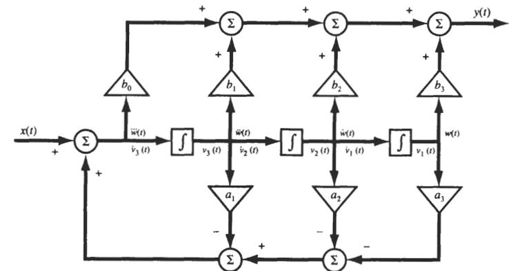
Fig. 7-16 Canonical simulation of the second form.
