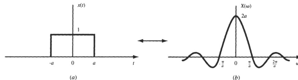
Fig. 5-16 Rectangular pulse and its Fourier transform.
