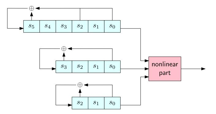
**Combination generators:** use multiple LFSRs and combine their outputs in some nonlinear way
