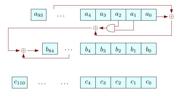
• Three FSRs (say A, B, C) of degrees 93, 84, and 111 (overall, the state is 288 bits long)
