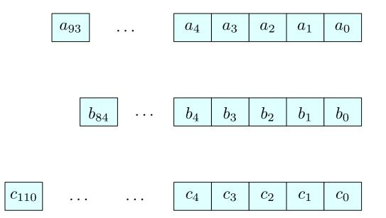
• Three FSRs (say A, B, C) of degrees 93, 84, and 111 (overall, the state is 288 bits long)
