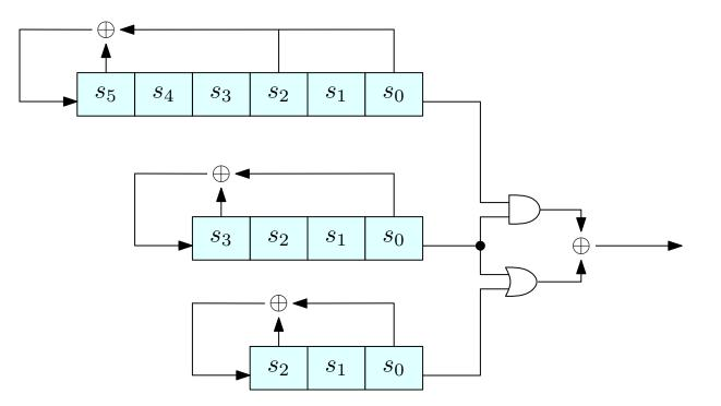
**Combination generators:** use multiple LFSRs and combine their outputs in some nonlinear way
