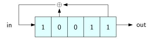
The content of the register is called the **state** of the register
