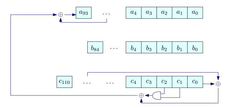
• Three FSRs (say A, B, C) of degrees 93, 84, and 111 (overall, the state is 288 bits long)
