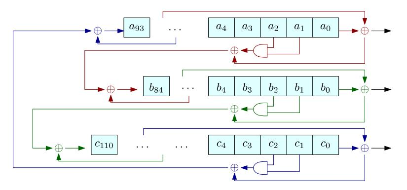
• The output of each FSR is the XOR of its rightmost bit plus the content of another register
