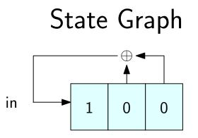
We can create a state graph G = (V, E) in which each vertex is a state, i.e.,  $V = \{0, 1\}^n \dots$ ... and there is a directed edge labelled  $y \in \{0, 1\}$  from st to st' iff Next(sf) = (y, sf').
