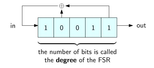
The value of the "in" line is the XOR of a subset of the bits in the register
