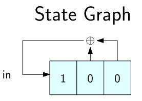
We can create a state graph G = (V, E) in which each vertex is a state, i.e.,  $V = \{0, 1\}^n \dots$
