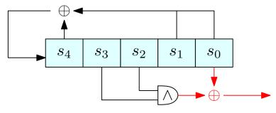
In the example:  $g(s_0, s_1, \ldots, s_{n-1}) = s_2 \wedge s_3$
