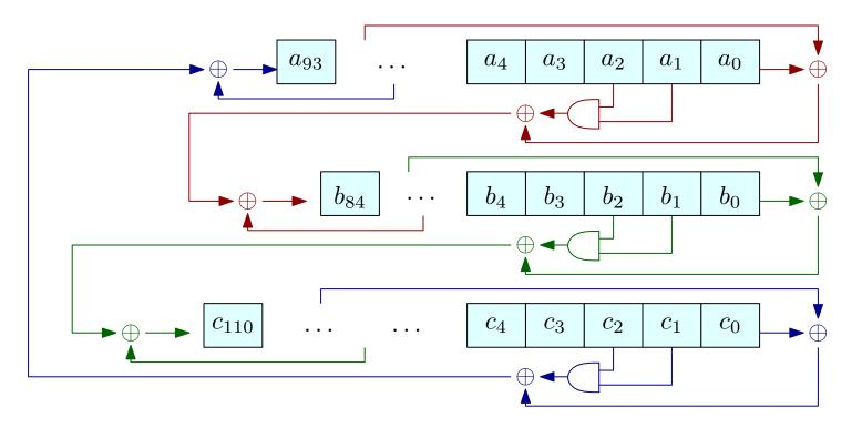
• Three FSRs (say A, B, C) of degrees 93, 84, and 111 (overall, the state is 288 bits long)
