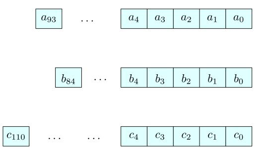
• Three FSRs (say A, B, C) of degrees 93, 84, and 111 (overall, the state is 288 bits long)
