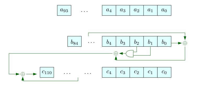
• Three FSRs (say A, B, C) of degrees 93, 84, and 111 (overall, the state is 288 bits long)
