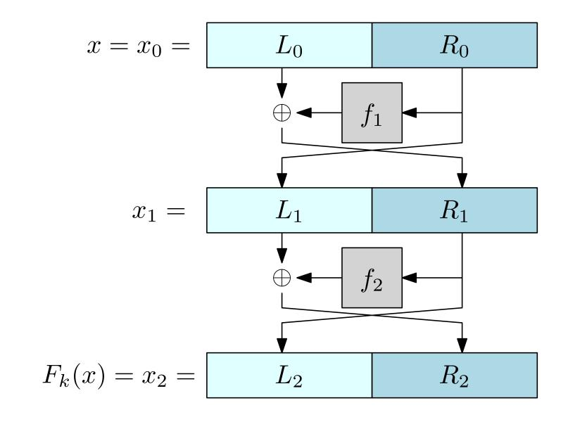
How can we exploit this? Pick  $R_0=R_0'$  This is easy to distinguish from a random function. E.g., pick  $L_0=0^{\ell/2}$  and  $L_0'=1^{\ell/2}$
