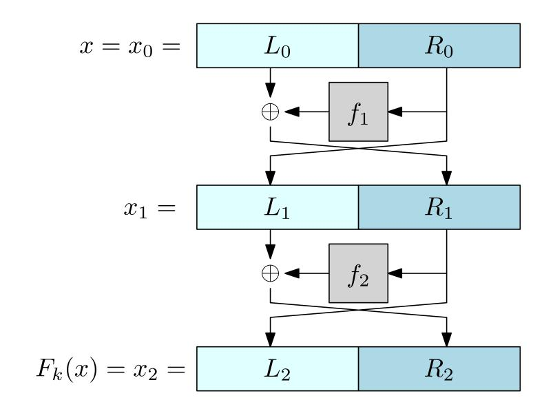
How can we exploit this? Pick  $R_0=R_0'$  This is easy to distinguish from a random function. E.g., pick  $L_0=0^{\ell/2}$  and  $L_0'=1^{\ell/2}$
