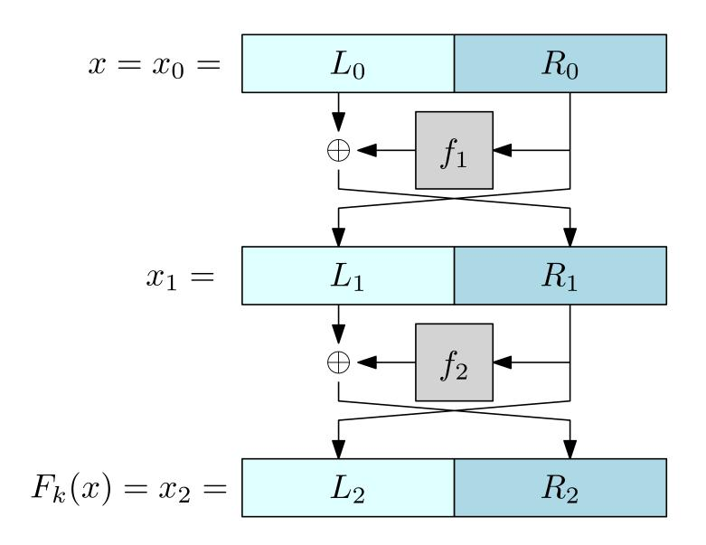
$$F_k(L_0 \parallel R_0) = L_2 \parallel R_2$$
