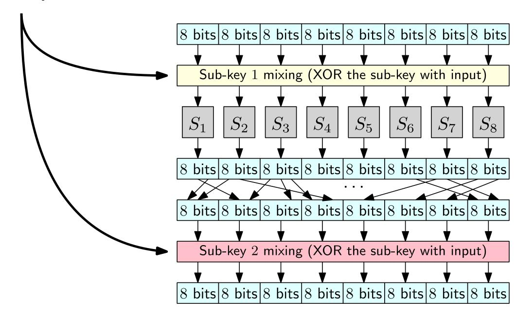
Consider now a **full** 1-round SPN (with the final key mixing step), in which the master key is just the concatenation of two independent sub-keys
